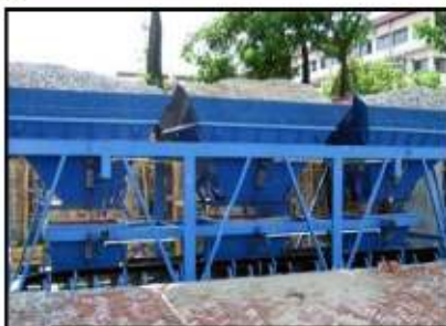
AGGREGATES STORAGE HOPPERS
